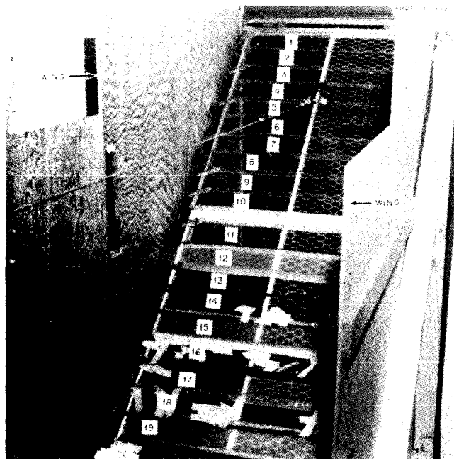
Fig. 6.1. A 6-foot KAP tested for durability at Oak Ridge. After 1000 hours of operation during which it pumped air through a room at a rate of 4000 cubic feet per minute (4000 cfm), there were only minor tears in the plastic flaps.
