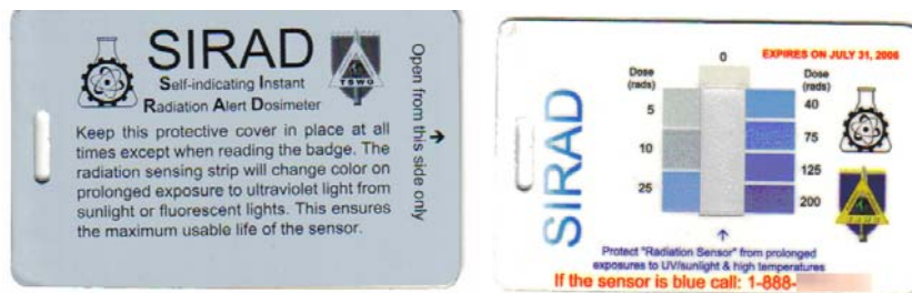
Figure 1. Front of SIRAD card. The image on the left shows a protective cover flap, and the one on the right shows the underlying SIRAD card with its radiation sensitive strip and color-matching scale. It was developed by Dr. Gordhan Patel, JPLabs ( www.jplabs.com ) with support in 2003-2005 from the Technical Support Working Group (U.S. Departments of Homeland Security, Defense, Justice, and State). Its early development (1995-1997) was supported by the U.S. Navy.
